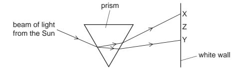
The dispersed beam is incident on a white wall between X and Y.
